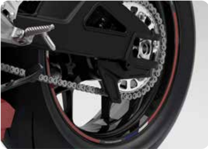
SPROCKET PROTECTOR 08P77-MKR-D10 Preventing objects from getting caught in the sprocket, this heavy-duty cover will not impair the bend of the swingarm. Designed to conform to circuit regulations, it also increases the Racing appearance of the Fireblade RR-R.
