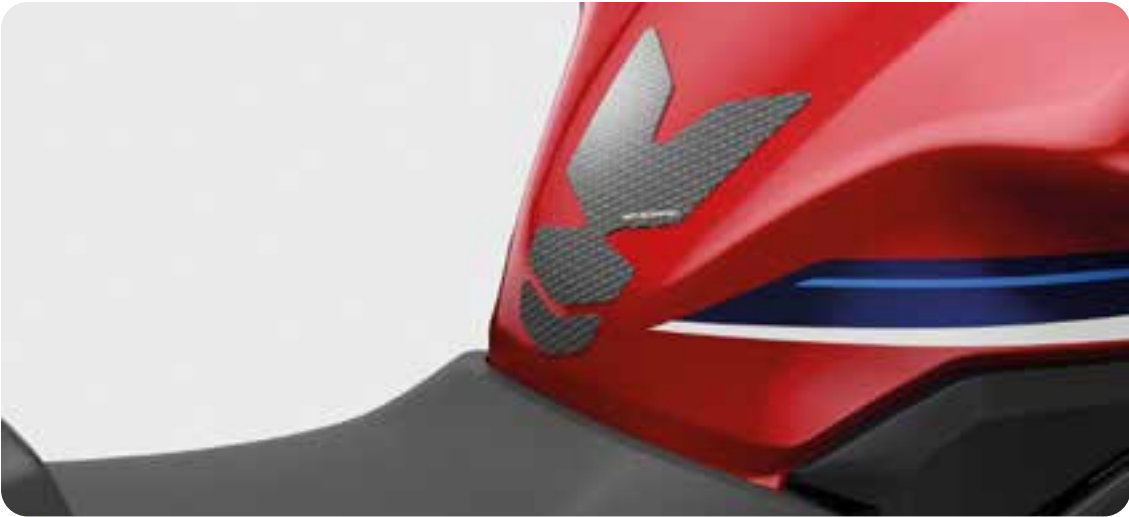
TANK PAD (CBR LOGO) 08P71-MKF-DK0 A distinctive arrow-shaped grey tank pad, showcasing the CBR logo, designed to safeguard your tank's paintwork from scratches and rubbing.
